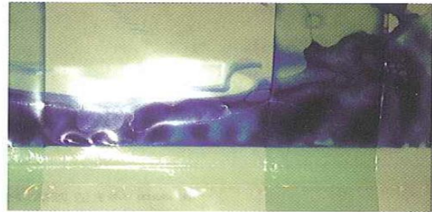
Fig. 3: Perfect seal seam (here: gusseted pouch sealed using hawo sealing device, test with hawo InkTest)
